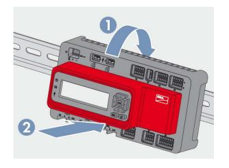
> Must attach to 35mm DIN rail at least 26cm (10 inches) long
